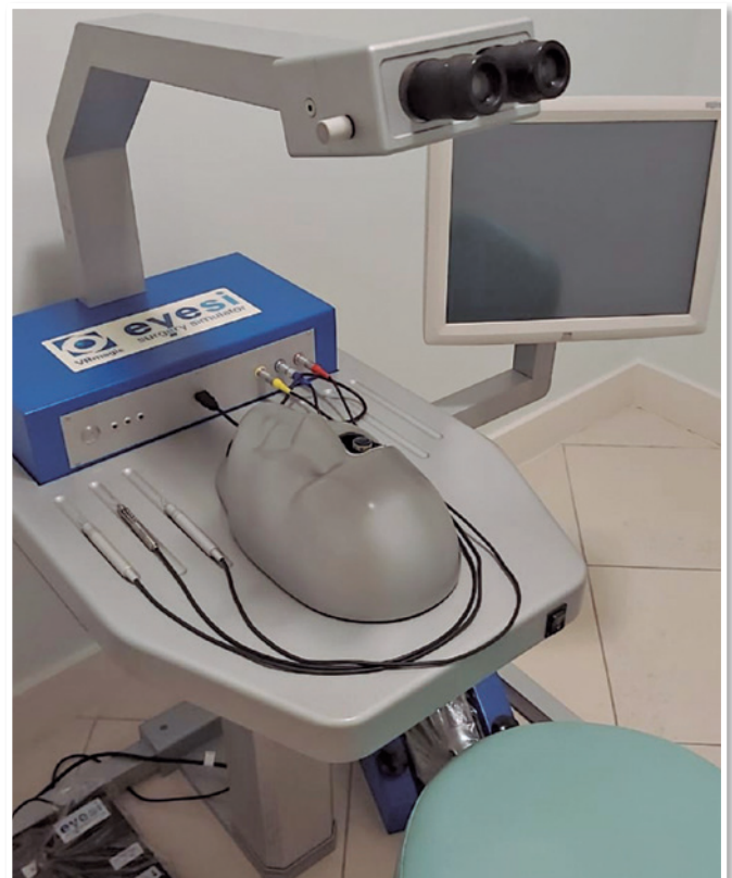
Figure 1. The Eyesi surgical simulator. The model has a mannequin with a model eye with three portable probes designed to use various surgical instruments.
